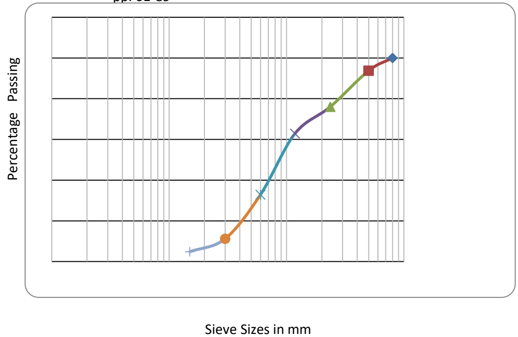
Figure 3.1: Fine Aggregate Sieve Analysis Graph
